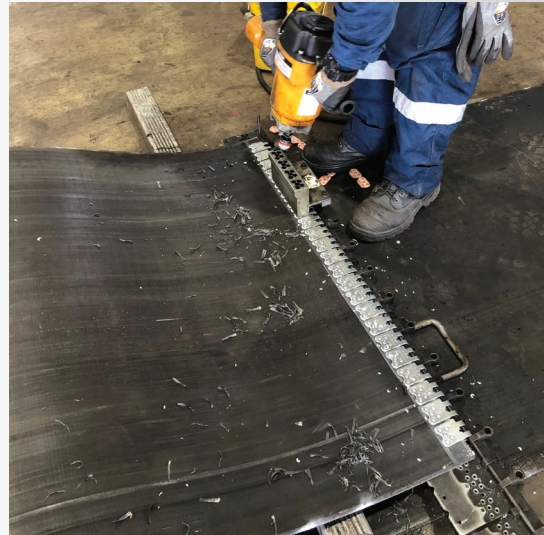
Stonebridge teaches the belt crew how to safely install fasteners with the Pneumatic Single Rivet Driver from Flexco.
